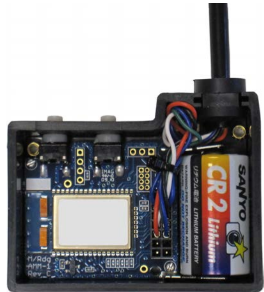
Gage Cable Connected to Command Mobile Module with ATZB Radio
