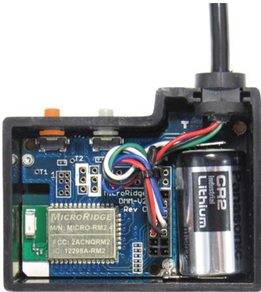
Gage Cable Connected to Command Mobile Module with RM2.4 Radio
