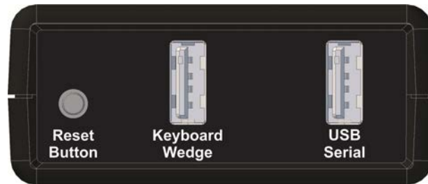
CAD Drawing of Wedge/USB Base Back Panel (Labels are shown for reference only)
