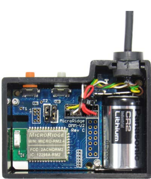
Gage Cable Connected to RS-232 Mobile Module with RM2.4 Radio
