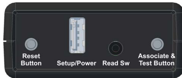
CAD Drawing of Remote Back Panel (Labels are shown for reference only)
