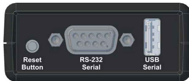
CAD Drawing of RS-232/USB Base Back Panel (Labels are shown for reference only)
