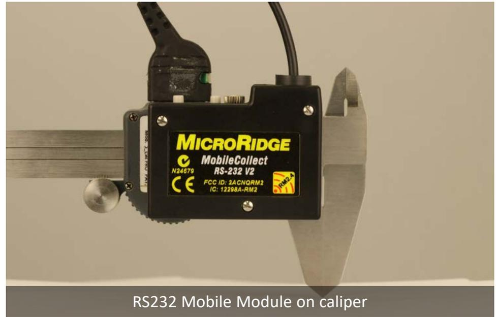
RS232 Mobile Module on caliper
