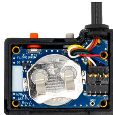
Mini EVO with M3 Connector (Left pins unused)
